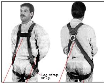
Chest strap drawn up tight Main body tightened to be comfortable Leg strap snug Fall arrest attachment dee or nylon loop high in center of back Strap under the buttocks
